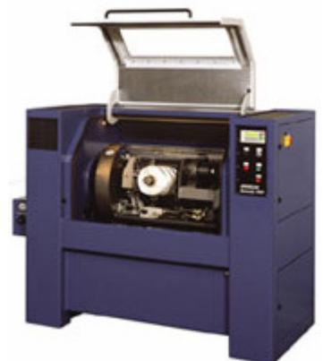
The ROBLON Tornado 300 is a two-for-one twister particularly suitable for production of rope yarns, industrial fibers, tying twine and baler twine, as well as for plying pre-twisted yarns.
